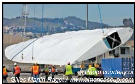
USA-17's 223-foot wingsail mast was removed from the hull for shipping.
