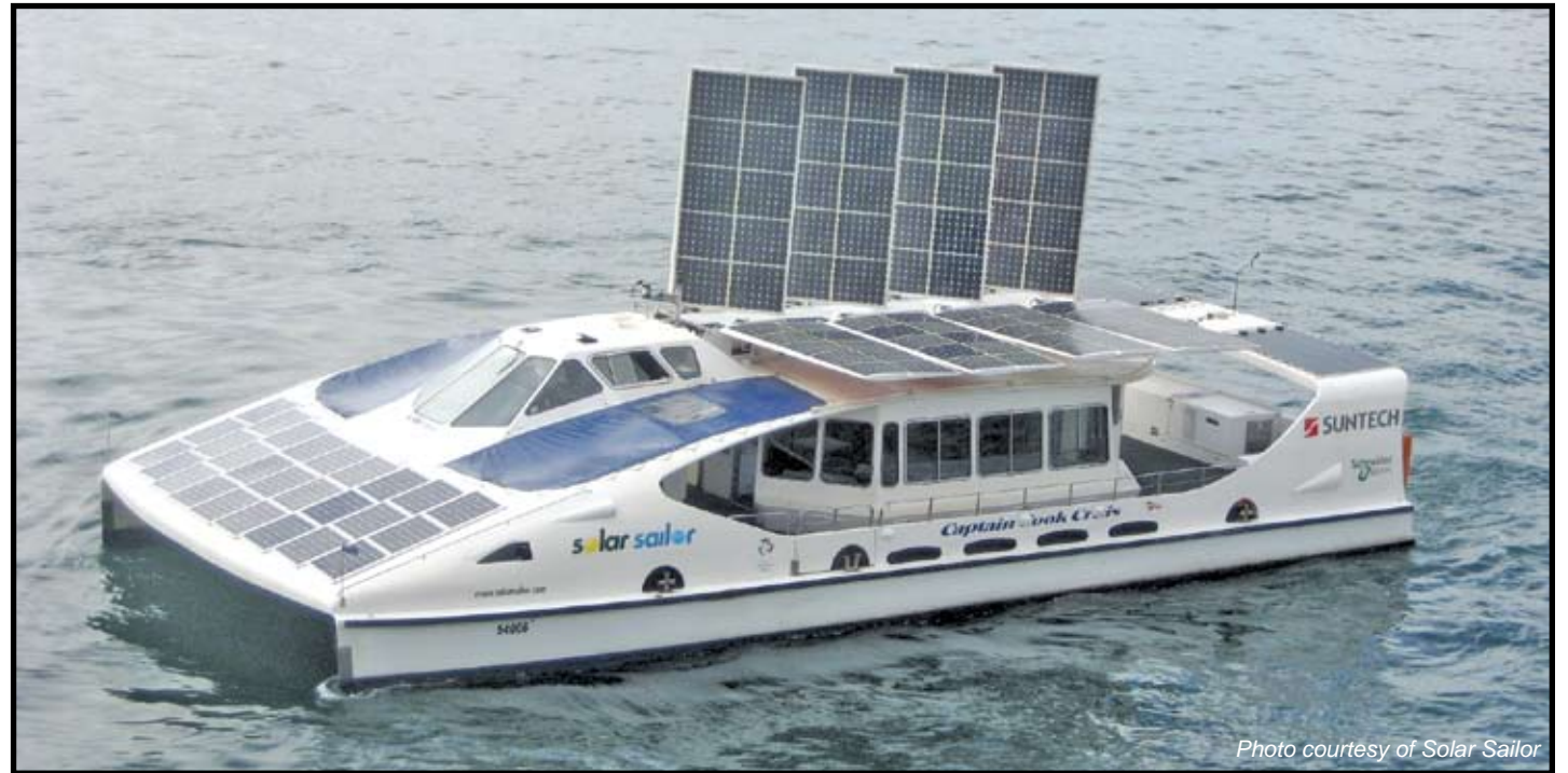
Solar ferries produced by Solar Sailor have been used for years commercially in Australia's Sydney Harbor.
