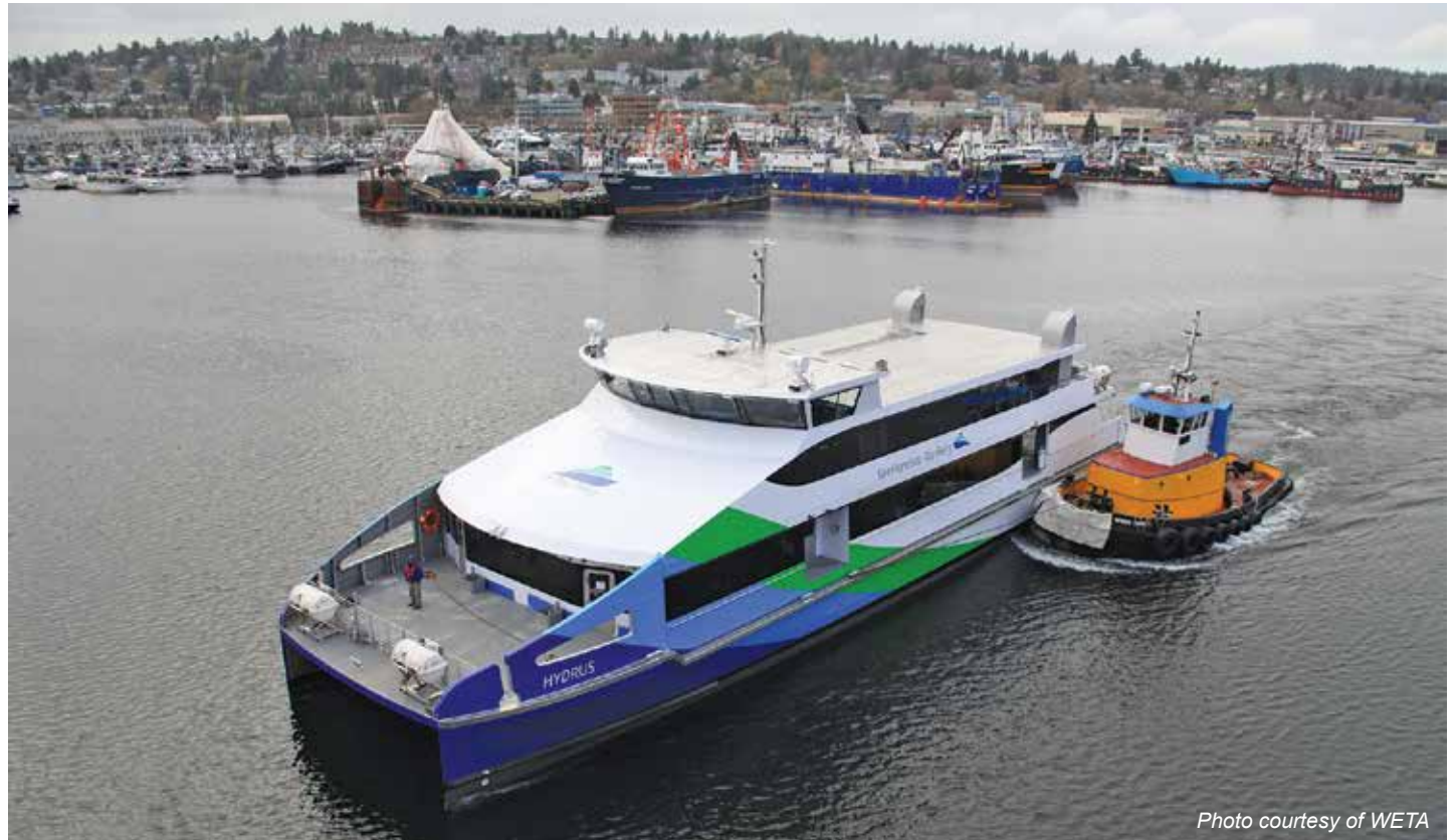
The newest boat in San Francisco Bay Ferry's fleet is the 135-foot Hydrus, with a capacity of 400 passengers and 50 bikes.
