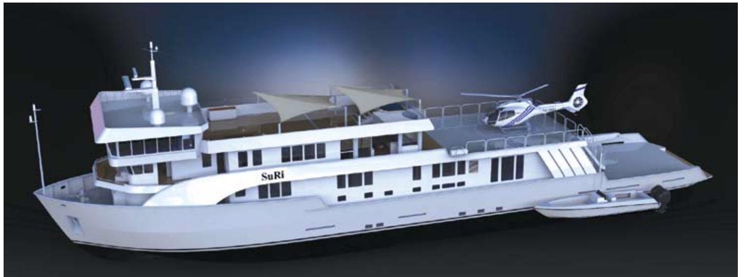
The model pictured above shows the expedition yacht SuRi with the 36-foot mid-body hull extension that is being added by Alameda's Bay Ship & Yacht.
