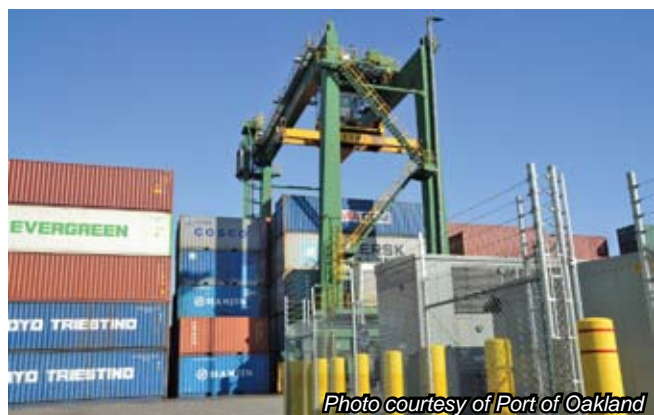
Photo courtesy of Port of Oakland The smaller rubber tire gantry cranes used to organize containers after unloading are still diesel-powered. A recent grant received by the port will allow for two of the cranes to be outfitted with a hybrid electric system.
