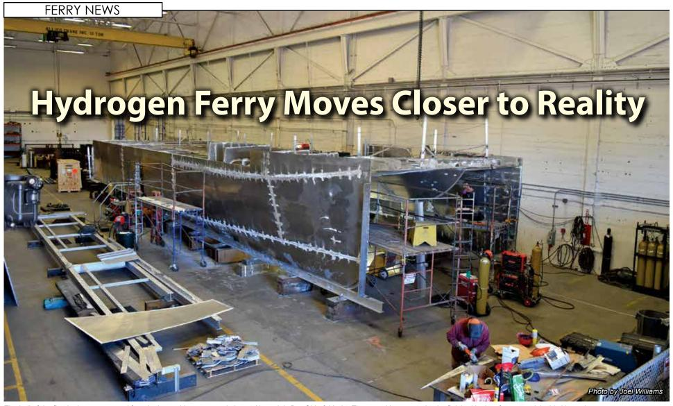
The hull of the first hydrogen-powered ferry in the world nears completion at Alameda's Bay Ship & Yacht. The vessel is expected to be finished in time for water trials this November.
