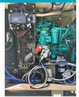
The new hybrid engines use much less fuel because they are used only to recharge the crane's batteries.
